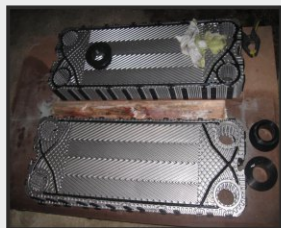
plate heat exchanger
